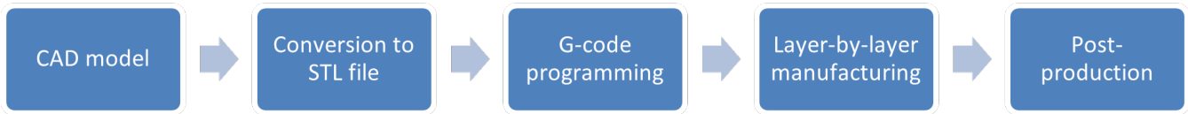
Figure 6. Steps in additive manufacturing.
