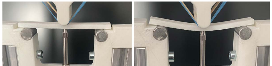
Figure 5. Specimen in the testing machine, unloaded (left) and loaded (right).
